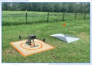
Photo of SVDN's DJI's Matrice 300 and lidar payload first flight at the Brandon IRS site.
