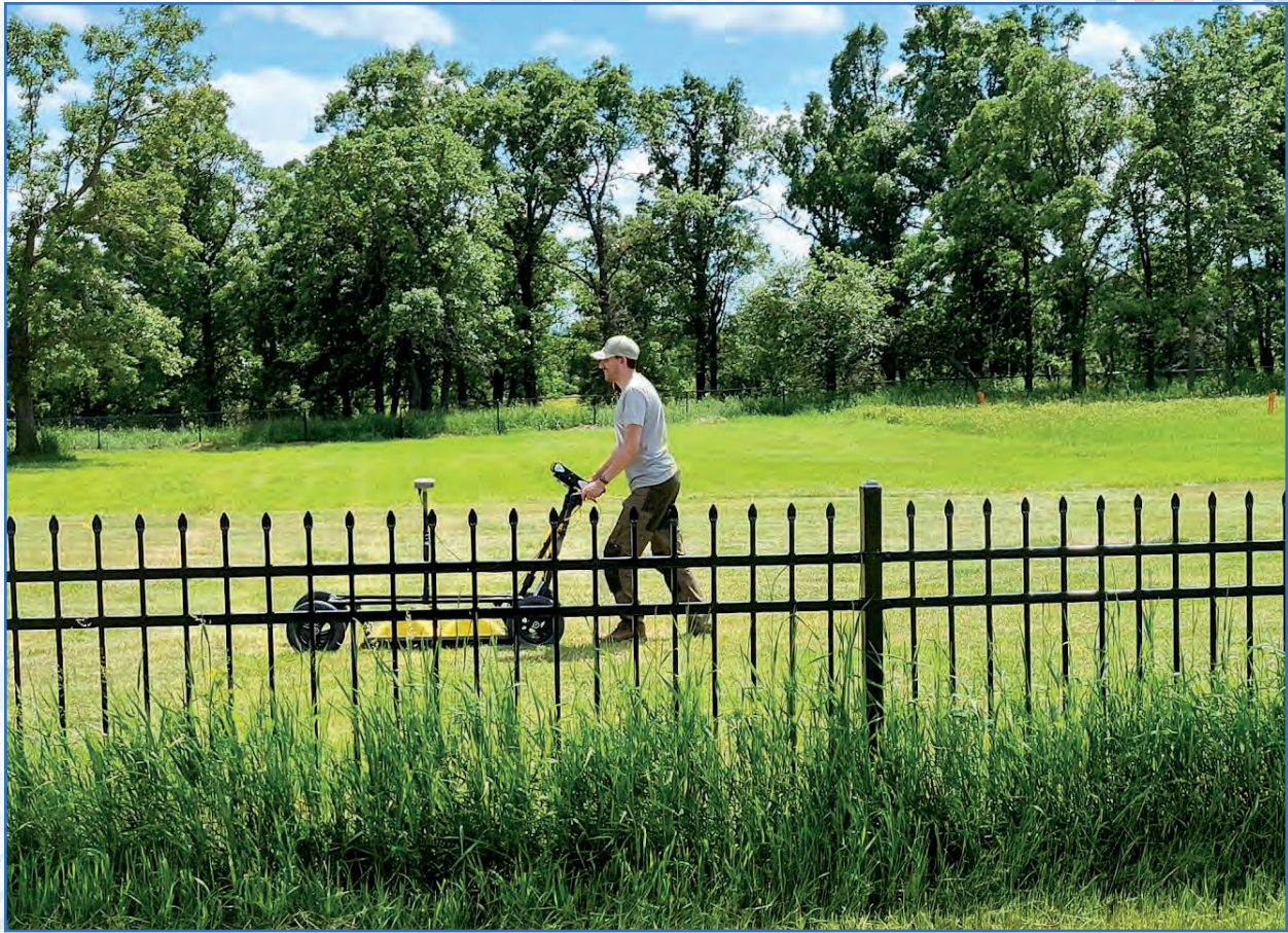
Christopher Mancuso conducting GPR Survey with 250 Mhz Antenna
