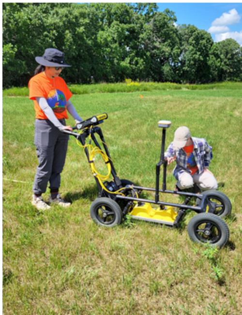
Left: Chris Mancuso & Kate Decter teaching a GPR acquisition workshop. Middle and Right: Ling Jin, Ashley Austin, and Chris Mancuso — calibrating the GPR prior to the survey and conducting the GPR survey.
